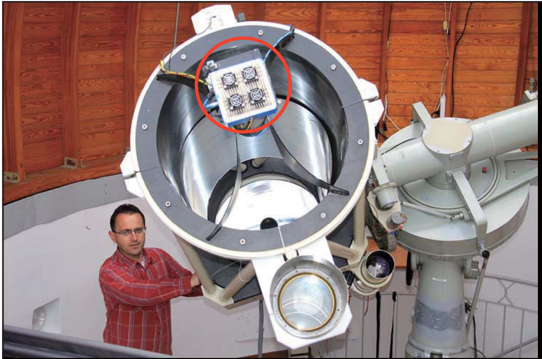
New system of photometric observations: The CCD camera was put in the main focus of the telescope Advantages: 1) larger field of view 2) less loss of light
