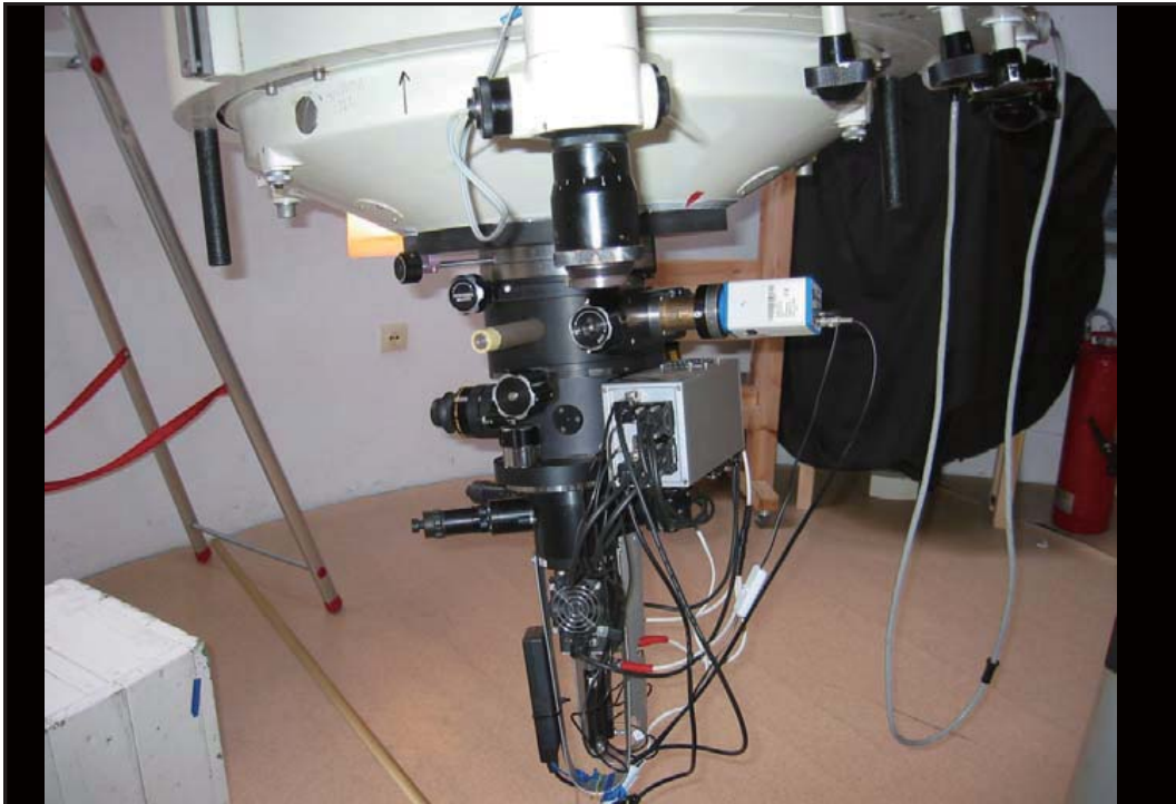
Three-channel photometer made by Astronomical Observatory in Vilnius (Lithuania) used at the 60 cm telescope of Mt. Suhora Observatory since 2005
